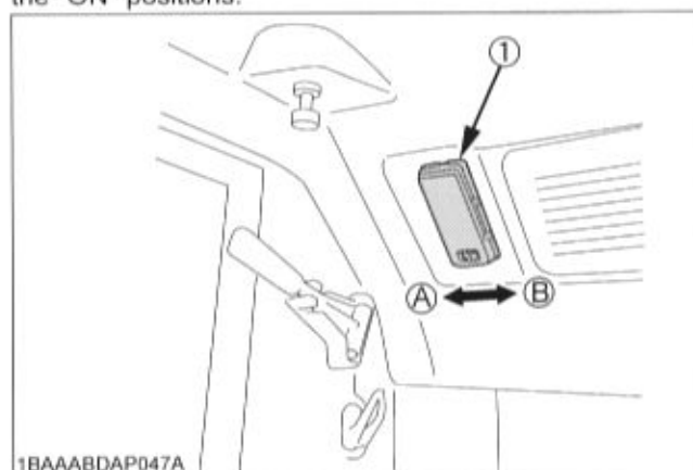
(1) Interior lamp (2) Interior lamp switch
